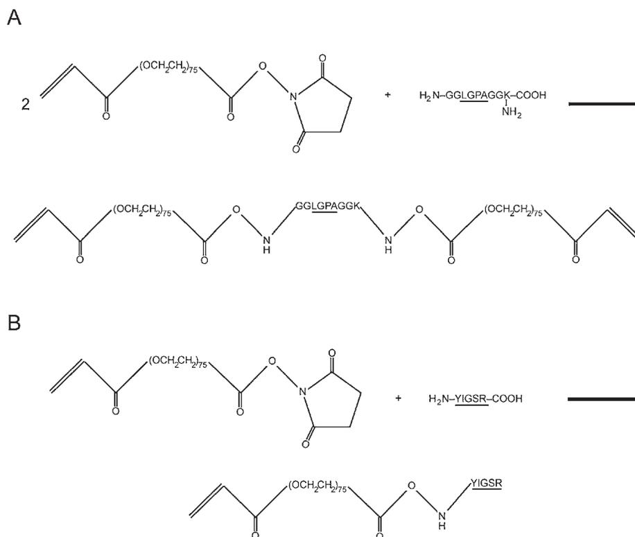
**FIG. 1.** (A) Coupling of collagenase-sensitive peptide, LGPA, with acryl-PEG-NHS to form a degradable hydrogel, ABA block copolymer, terminated in acrylate groups for photopolymerization. (B) Coupling of cell-adhesive peptide, YIGSR, with acryl-PEG-NHS to facilitate preadipocyte binding to hydrogel.<sup>21</sup>
